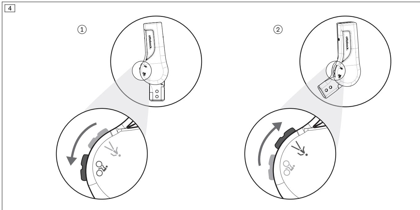
For certain activities (such as cycling), it may be beneficial to temporarily unlock the orthotic knee joint. Mechanical unlocking of the orthotic knee joint is indicated by the symbol of a cyclist (switch to "🚴").
