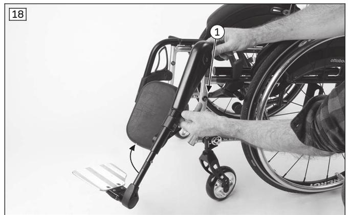
**Removing the leg supports – amputation leg support on the Avantgarde DF version V**
