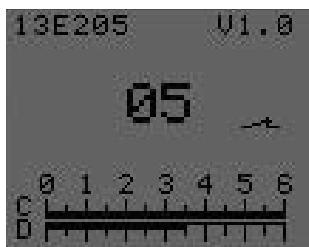
Switching between gripping function and rotation is performed by impulse switching, which means that the control signal must quickly exceed the upper threshold and then quickly subside. See section 5.2 "Switching". In addition, a time control feature can be used to switch back to the gripping function. The switch-back time is set using the 757T13 MyoSelect. The respective setting can be read on scale C on the MyoSelect's display.
