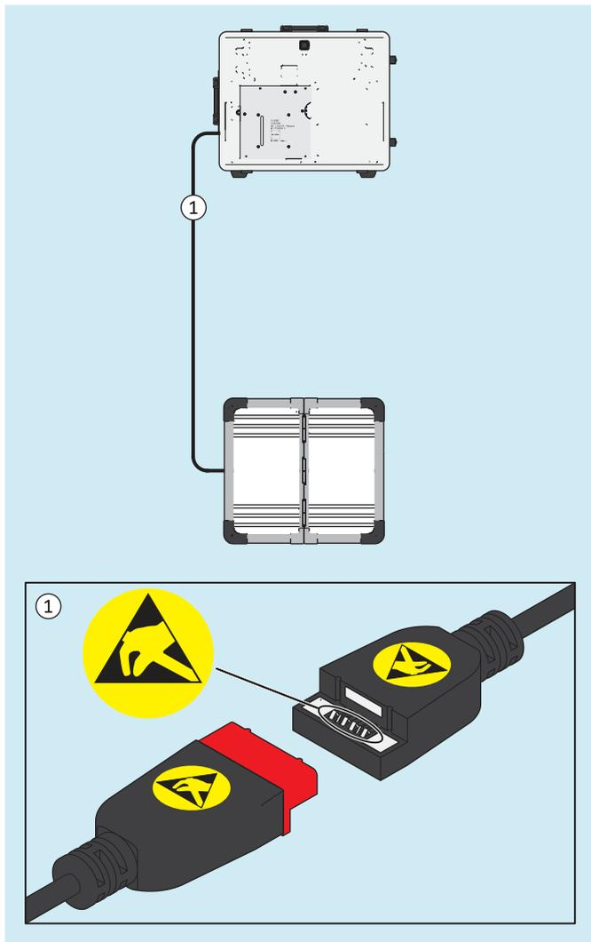
► **NOTICE!** To prevent electrostatic discharge, be sure to maintain a sufficiently safe distance between your fingers and the contacts of the magnetic USB coupling (> 10 mm).
