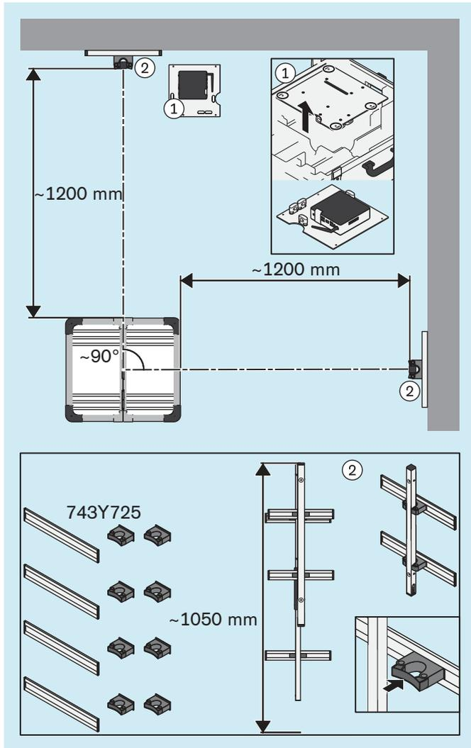
Instead of the standard setup for the camera stands in the holders of the upper and lower case sections, the upper sections of the camera stands may be installed in the 743Y725 wall holders.
