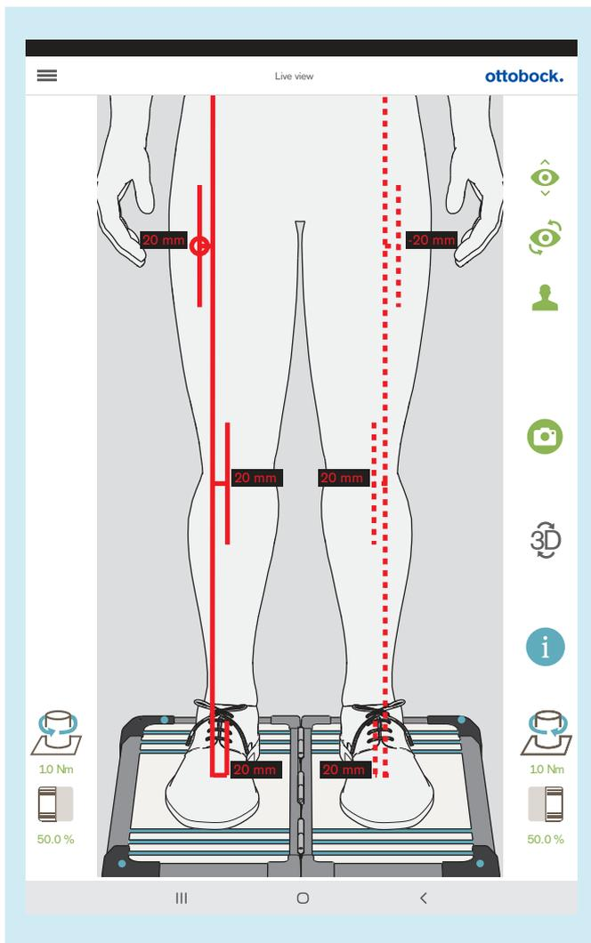
The illustration shows how the alignment recommendation for the frontal view from the sample instructions for use for the prosthetic knee joint can be readjusted and checked with several auxiliary lines in the live view.
