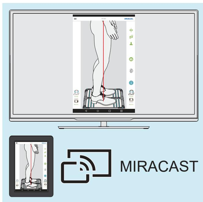
The tablet screen can be transferred to and displayed on another device over a wireless connection using Miracast, a peer-to-peer radio screencast standard (for example a television screen or monitor with Miracast HDMI dongle or a computer with Miracast adapter).
