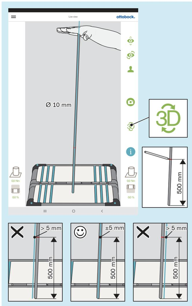
Calibration in this section serves to check the measuring accuracy of the product against specified tolerances.
