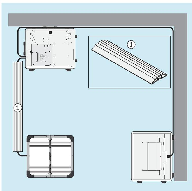
Optional cable protectors can be used to reduce the risk of tripping and damaging the cables.
