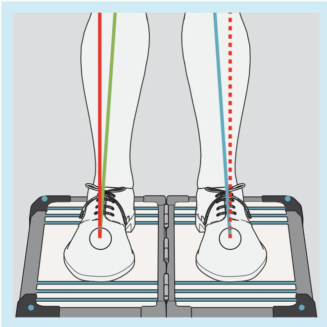
The force transmission points (bottom ends of the load lines) are in the same place whether 3D mode is activated or deactivated (see markings in the illustration). Simultaneous display is not possible in the app.
