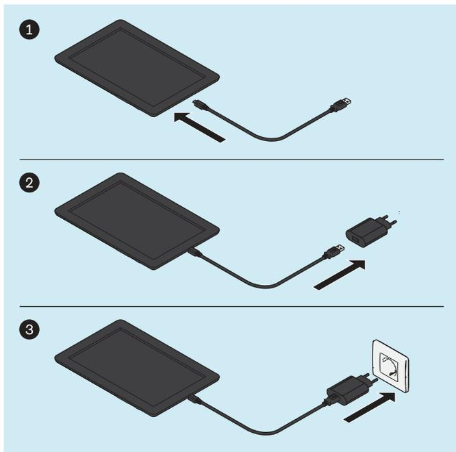
► **CAUTION!** To protect against leakage currents, the patient is not permitted to come into contact with the tablet during charging, directly or indirectly (for instance through another person).
