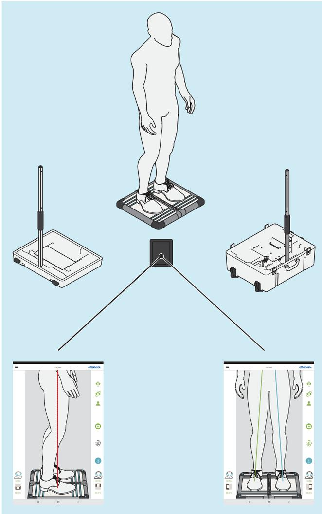
The 3D L.A.S.A.R. Posture is a measuring device intended for verifying and optimising the static alignment of prostheses and orthoses together with the patient.
