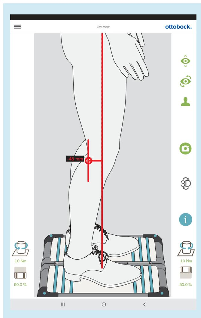
The illustration shows how the alignment recommendation for the sagittal view from the sample instructions for use for the prosthetic knee joint can be readjusted and checked with an auxiliary line in the live view.
