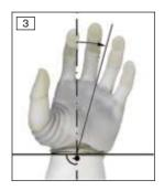
The Michelangelo Hand Transcarpal is designed in such a way that the hand is positioned in a slightly flexed (**see fig. 2**), ulnar deviation (**see fig. 3**) position when the lamination ring is mounted at a 90° angle to the socket axis (**see fig. 1**).
