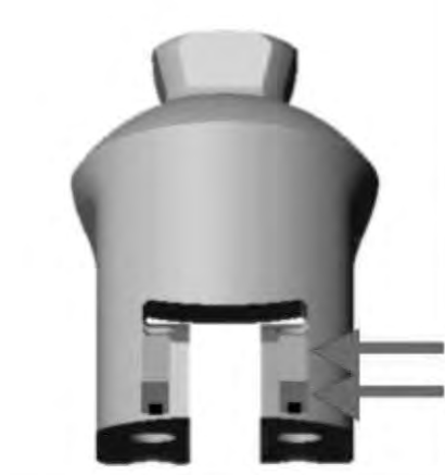
Shim Shim adjustment screw
