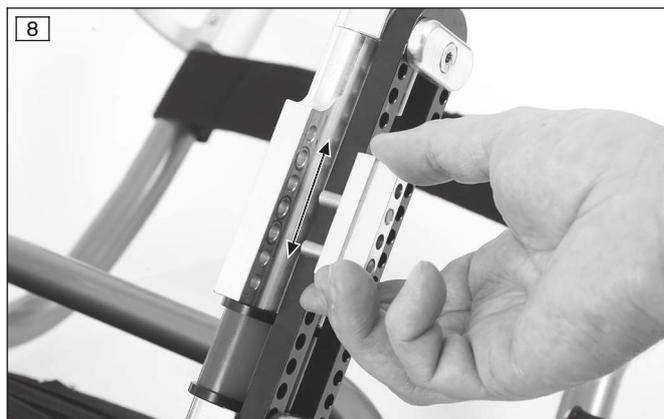
**6.2.3 Adjusting the drive wheel camber**
