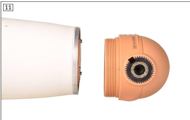
12) Screw the elbow joint into the upper arm.
