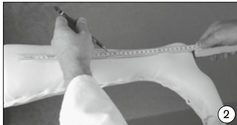
Please subdivide the model into two parts to determine the fixed area and the movement area for the carbon fiber spring. Measure the distance from the medial tibial plateau to the floor and mark the middle (see sketch 3).
