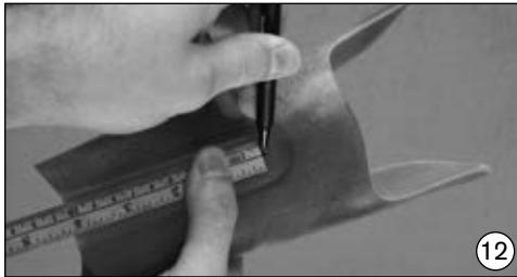
Mark the bore holes on the calf piece. A ruler can be used to mark the middle.
