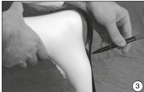
Trace the carbon fiber spring on the bottom of the foot. The length of the carbon fiber spring extends up to approx. 20 mm in front of the roll-over area when viewed from the calcaneus. Then determine the calf length of the carbon fiber spring. The end of the carbon fiber spring reaches up to 20 mm below the flexion cutout.
