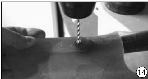
Use a 4 mm drill for M4 to make the hole in the polypropylene. Use a 5 mm drill for M5.
