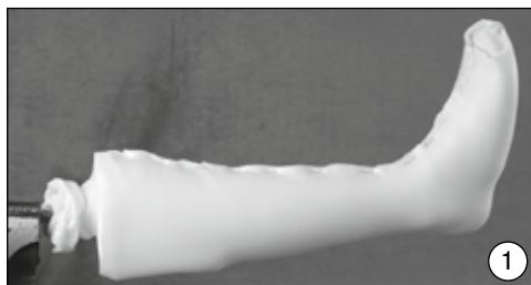
Pull layer of perlon stockinette over the plaster model and fabricate Pedilin insert (617S3=W5).
