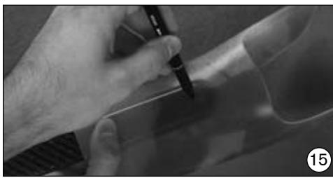
Hold carbon fiber spring below polypropylene and mark the places for the bore holes on it.
