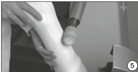
To adapt the carbon fiber spring to the lower leg, the insert must be mounted on the appropriate places and sanded. If need be, cavities must be filled in.
