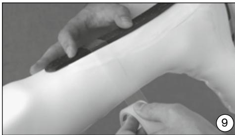
Prepare model for vacuum forming. Use the Polyethylene Adhesive Tape (627B4) to attach the carbon fiber spring to the model above the ring/span and below the calf. Pull 1 Perlon stockinette over the model.
