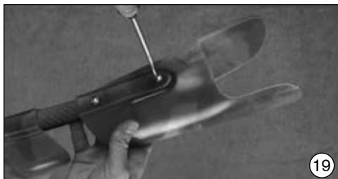
Screw together carbon fiber spring with the provided 501S86 Niro Countersunk Head Screw and the provided 507U9 Rosette Washers. The rosette washers prevent you from pressing the screws into the polypropylene and ensures that there is a large contact surface.
