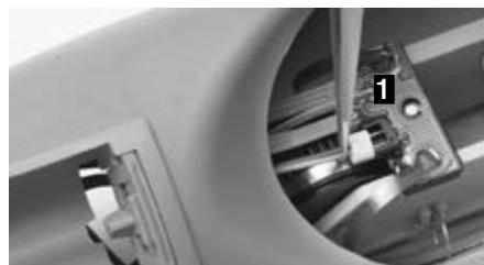
After mounting the battery box, plug the battery connection cable 13E51=2/4 into the circuit board **[1]** of the forearm cable. (The circuit board is attached to the AFB.)
