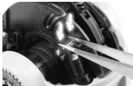
...and snap it in onto the projecting metal axle [1].
