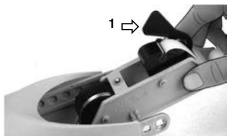
Lock the band cam to the extension stop using the fixation fork [1].
