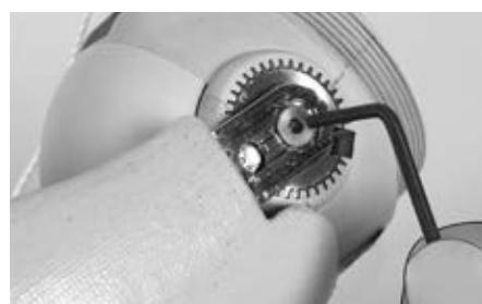
Unscrew the two elbow joint attachment screws.
