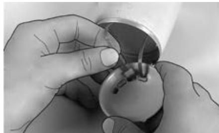
Plug in the cables, being certain they are fully inserted into the connectors.
