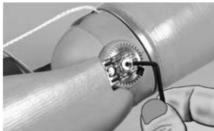
Apply one drop of Loctite 243 or equal to the two elbow joint attachment screws and tighten them **evenly**.
