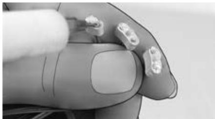
Remove all dummy plugs from the electronics housing.
