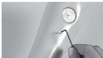
Tighten the AFB mounting screws, located in the forearm.
