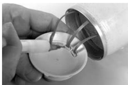
Protect these connections from moisture damage by applying 633F11 silicone grease liberally to the top of the connectors.
