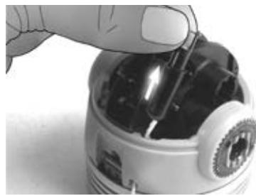
Take off the cord clamp (by cutting at the terminal knot) and remove the telescopic spring.
