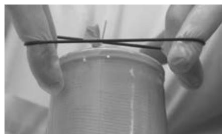
Laminate the socket. Stretch rubber ring and place around the ungelled resin beneath the lamination protection cap.
