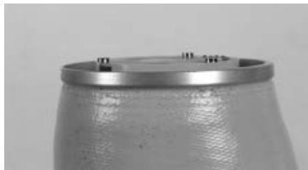
The illustration shows that the plate and brim of the lamination ring are level with each other.
