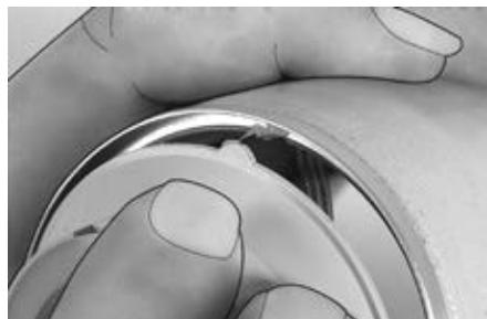
Push the electronics housing, including the installed wires, into the lubricated lamination ring and press **firmly**.
