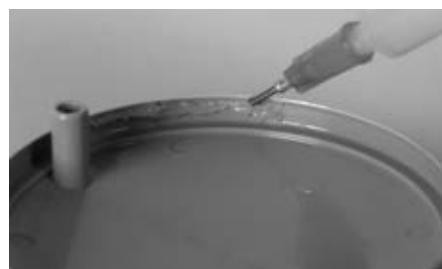
Lubricate the lamination protection cover with 633F30 special grease.
