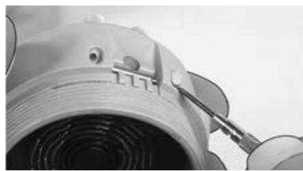
Remove the dummy plug and insert it into the hole on the other side.
