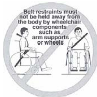
Improper Positioning of Belts on Occupant
