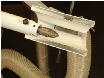
729W3=3 Râpe (pointu) ø30mm longueur 80mm M16
