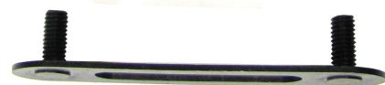
Part Number BR5001 Stud Plate (Inside of Shell) Use: 10mm hex socket or wrench Torque Specs: 117 in-lbs/ 13.2 N-m
