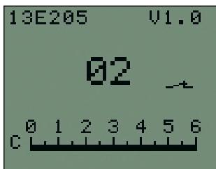
Switching between gripping function and rotation is performed with Cocontraction. See section 5.2 "Switching". In addition, a time control feature can be used to switch back to the gripping function. The switch-back time is set using the 757T13 MyoSelect. The respective setting can be read on scale C on the MyoSelect's display.
