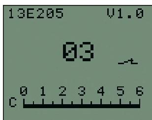
Switching between gripping function and rotation is performed with safety Cocontraction. See section 5.2 "Switching". In addition, a time control feature can be used to switch back to the gripping function. The switch-back time is set using the 757T13 MyoSelect. The respective setting can be read on scale C on the MyoSelect's display.
